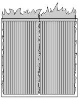
Figure 21 - Incorrect Burner Flame Pattern
